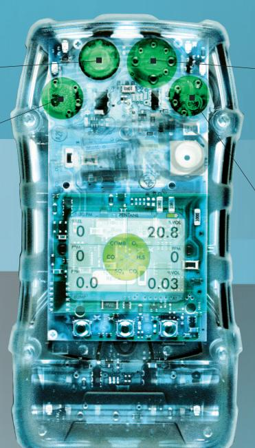
MSA XCell SO<sub>2</sub>, Cl<sub>2</sub>, or NH<sub>3</sub> Sensor
